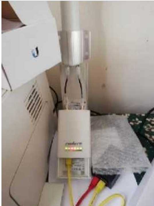
Figura 18: Antena Ubiquiti AirMax Omni+ Rocket M5
